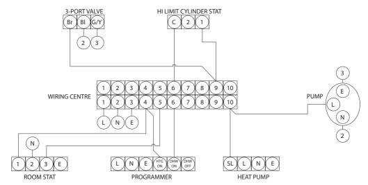
If the 3-port valve itself has not been fitted to building regulations to isolate the heat source from the unvented hot water tank in event of failure, a safety 2-port valve MUST be fitted on the flow into the cylinder coil and controlled via the high limit thermostat provided in the unvented kit, example wiring diagram for this is seen opposite.
